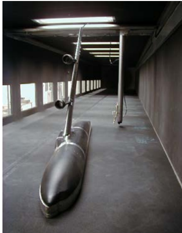
Transport aircraft half model configuration mounted in closed wind tunnel test section
