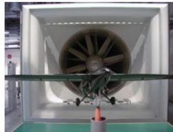
Figure 16-3: Versions of wind tunnel models (full, half-span) and test section installations.
